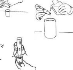
Swirl the meter once and when the reading in the display window stabilises, read the result while the electrodes are still immersed in solution.
